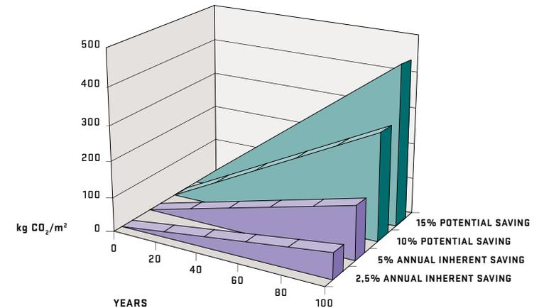
Lifetime consequences of small annual improvements in energy savings. Note: the inherent savings come automatically with a heavyweight building. The potential savings are obtained if the building and installations are specifically designed for maximum energy efficiency.
