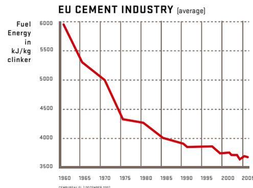
Cement manufacturing: the underneath chart indicates the reduction in fuel energy consumption from 1960 to 2005 (CEMBUREAU).
